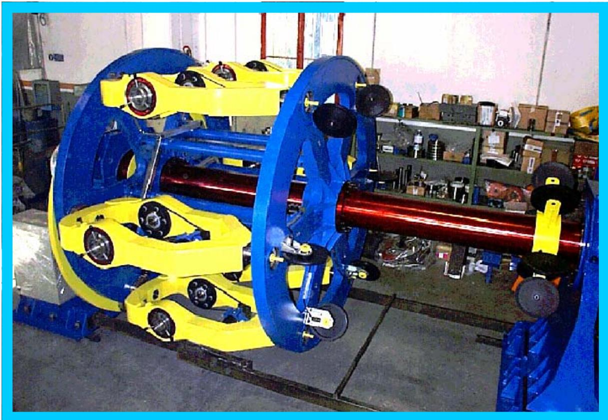
CAGE À 6 BOBINES AVEC DETORSION 100%.
